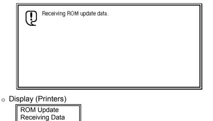
10. Once the machine has received the entire firmware module file, the firmware update starts automatically.
